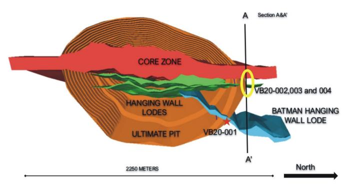
The plan view above shows the interpreted location of the Batman North Extension. VB20-002, -003, and -004 intersected the Batman North Extension at the predicted location and encountered a thicker mineralized zone than anticipated.
